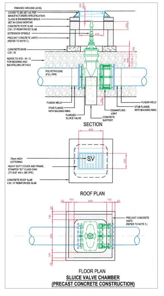
SLUICE VALVE DETAILS (scale 1:20) REFER TO IRISH WATER DRAWING STD-W-15 FOR CONSTRUCTION DETAIL.
