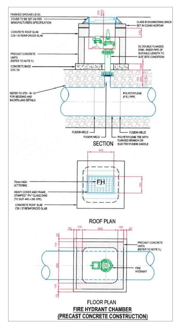
FIRE HYDRANT DETAILS (scale 1:20) TO IRISH WATER DRAWING STD-W-18. FOR CONSTRUCTION DETAIL.
