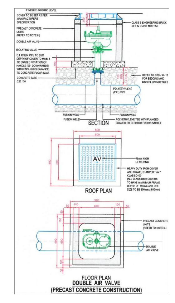
AIR VALVE DETAILS (scale 1:20) REFER TO IRISH WATER DRAWING STD-W-22 FOR CONSTRUCTION DETAIL.
